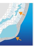
Left: gelcoat with air bubbles and non polymerised resin due to manufacturing defects.
