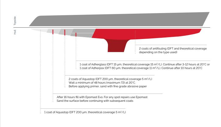
WE RECOMMEND: launching the boat a minimum of seven days after application of the final coat of Aquastop. ATTENTION: if the maximum recoating times are exceeded, always sand before continuing with the coating system.
